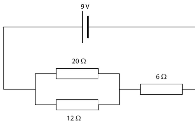
i) Calculate the current in the  $20 \Omega$  resistor.
