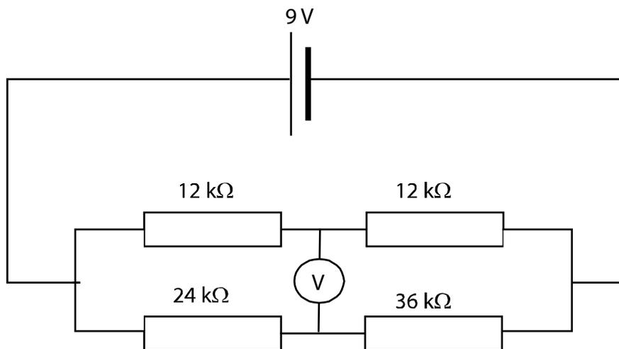
i) Calculate the potential difference displayed on the voltmeter.
